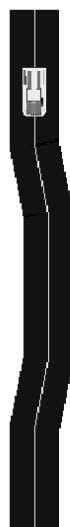
Fig. 2. Desired trajectory defined within the simulation software. Tracked vehicle can be seen on the top side of the figure (road strip is 7 m wide)
