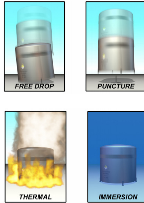
Fig. 3. Representation of Type B packages tests
